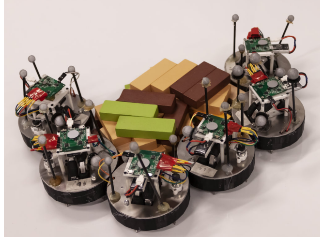
Fig. 1: The robots are collaboratively transporting an object with complex shape through caging. By magnetic docking with each other, robots can better maintain team formation to exert enough caging force while achieving omnidirectional movements for smooth transportation.
